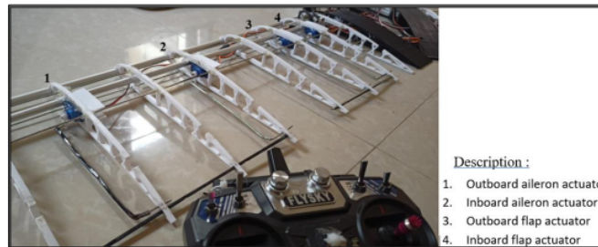
Figure 5. Servo actuator mounting configuration on rib morphing wing
